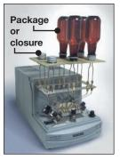
Package testing capability allows for package component or complete package testing.
