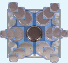
With the optional package adaptor, six packages may be tested simultaneously.
