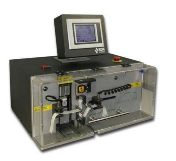
Heat seal applications are constantly evolving to meet the challenge of **higher specification materials and faster production methods**. Determination of hot tack performance requires a test method that provides **repeatable results**, free of operator interference. The falling weight principle or the spring test are difficult to regulate and only suited for rough pass/ fail evaluations.
