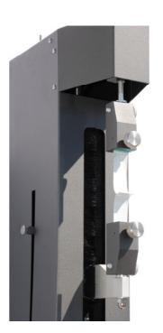
The SST-3XS Seal / Tensile Tester has been developed as a highly specialized machine to measure accurate low loads in tension and compression up to 50Kg (500N). The machine is ideal for seal strength measuring and general tension and compressive testing as required by the packaging, plastics and paper industries.
