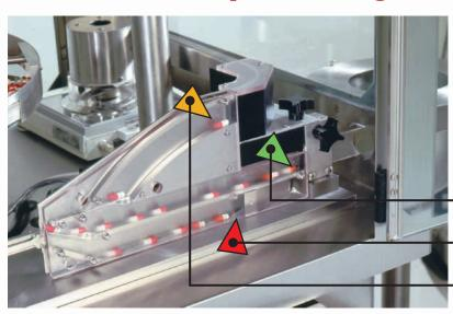
The high-speed sensor featured in the VERICAP® 4000 is capable of weighing capsules at speeds as high as 132,000 capsules per hour. To ensure precision, the VERICAP 4000 sensor re-zeros itself between every capsule weight measurement.
