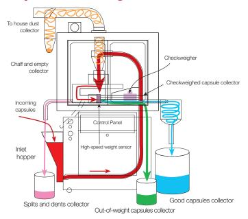
Incoming capsules from encapsulator or drums. Empties, chaff, halves, are removed and collected. Splits, dents, and other jams are cleared and collected. Out-of-weight tolerance capsules are rejected and collected. "Good" capsules are collected.
