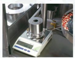
The VERICAP 4000 checkweigher provides a built-in analytical balance for a gravametric weight check of a capsule. This capability automatically makes minor adjustments to the VERICAP 4000 system calibration should it become necessary during the run. This ensures maximum precision and traceability. These checkweighed capsules are collected separately and are not returned to the batch population. The frequency and number of capsules checked is adjustable.
