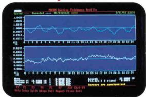
Two test runs (ie. substrate and coated substrate) can be measured to automatically determine coating thickness. The top half of the screen graphs both the coated and uncoated substrate, while the bottom half of the screen graphs the coating itself. By using a different scale on the coating profile, much higher resolution is possible.
