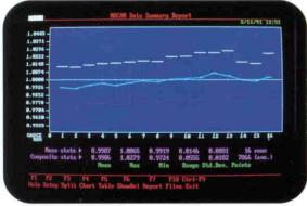
No-nonsense SPC capabilities include an  $\overline{X}$  and R chart on numerous test runs. Each test run (or sample) is depicted by a single verticle line. The top and bottom points of this line represent the upper and lower most gauge readings taken from this sample. Mean thickness is displayed as a series of dots connected by a line, while pertinent summary data is displayed below the screen. Data can be displayed in either table or chart form or a combination of both.
