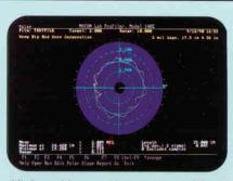
High and low spots on a blown film die are easily pin-pointed with the new Polar Graphics Profiles.
