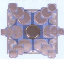
With the optional package adaptor, six packages may be tested simultaneously.
