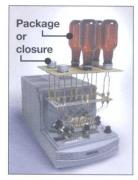
Package testing in accordance with ASTM F-1307
