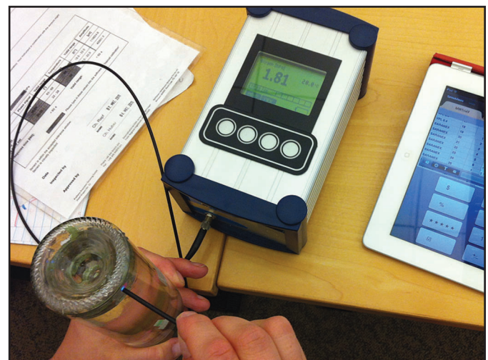
Figure 4. NOMASense O 2 Trace (Presens-Fibox 3LCD trace v 7 oxygen analyzer using Pst6 oxygen sensing ports (range 0–1.8 mg/L and 0–4.2% O 2 )).
