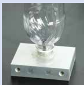
Container Transfer Unit (CTU) Allows conditioned packages to be easily transferred to the testing rack
